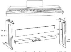
1-1 to 1-4 Round head knob screws M6X20 (4)2-1 to 2-4 screws M6X15 (4)
